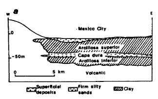
Fig. 1 An east-west section through Mexico City subsoil<sup>1</sup> (a), and a typical cross-section and soil profile in Bucharest<sup>8</sup> (b).
