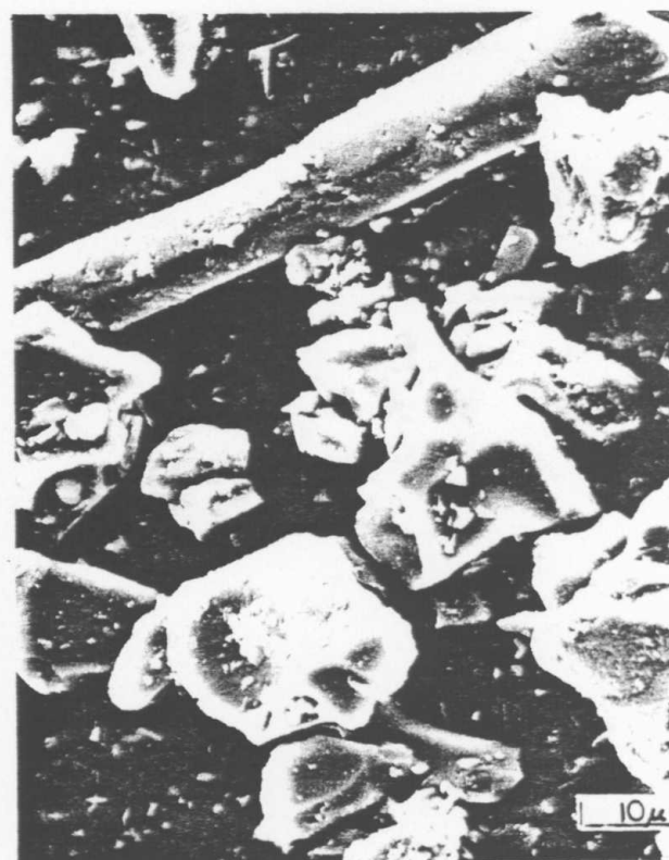
Fig. 3. Elongated hypersthene crystal (0.07 mm in length) among glass shards, \times 1,280 , SEM photo.
